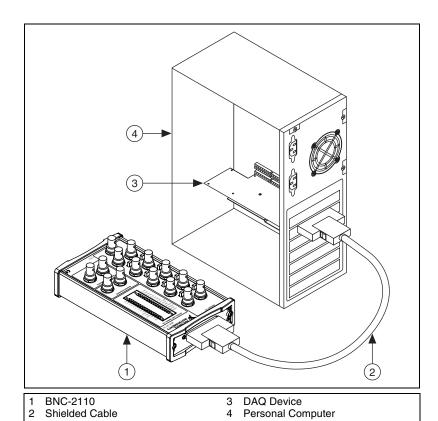
Figure 1. Connecting the BNC-2110 to Your DAQ Device
